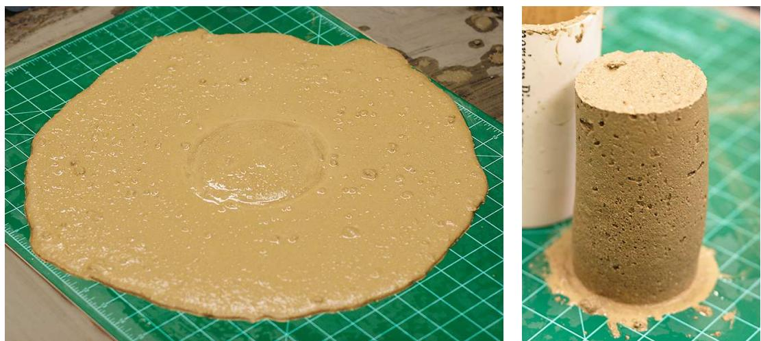
**Figure A.4** Comparison of slump-flow results for FRCA-based CLSM at high (left) and low (right) volumetric paste percent.
