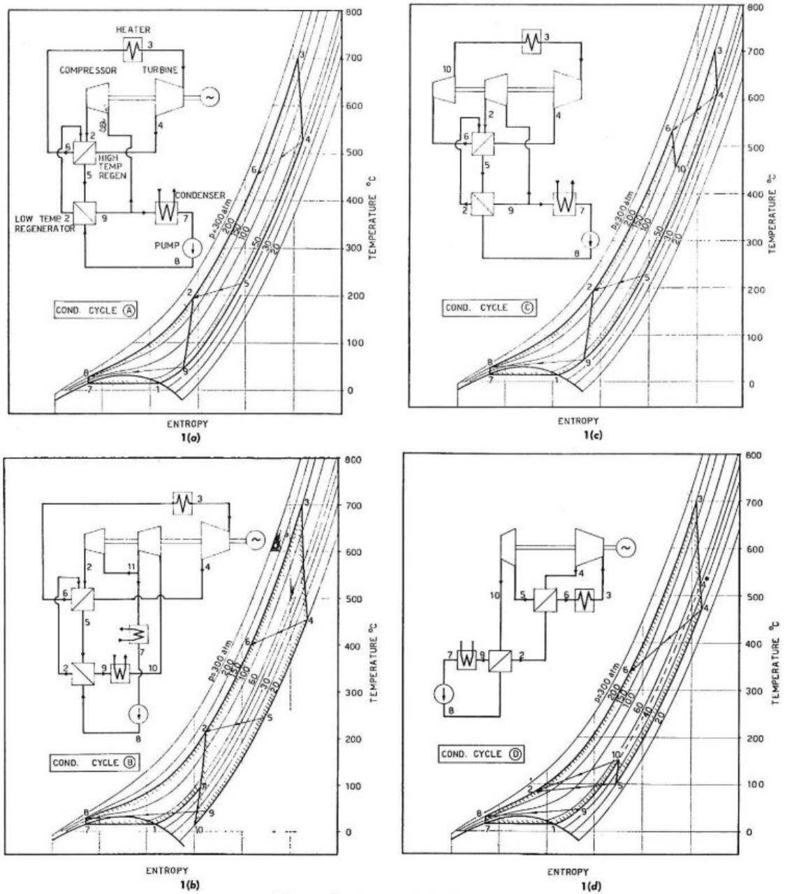
Figure 5.5: Supercritical Carbon Dioxide cycle configurations by Angelino. Source:Angelino [1968]
