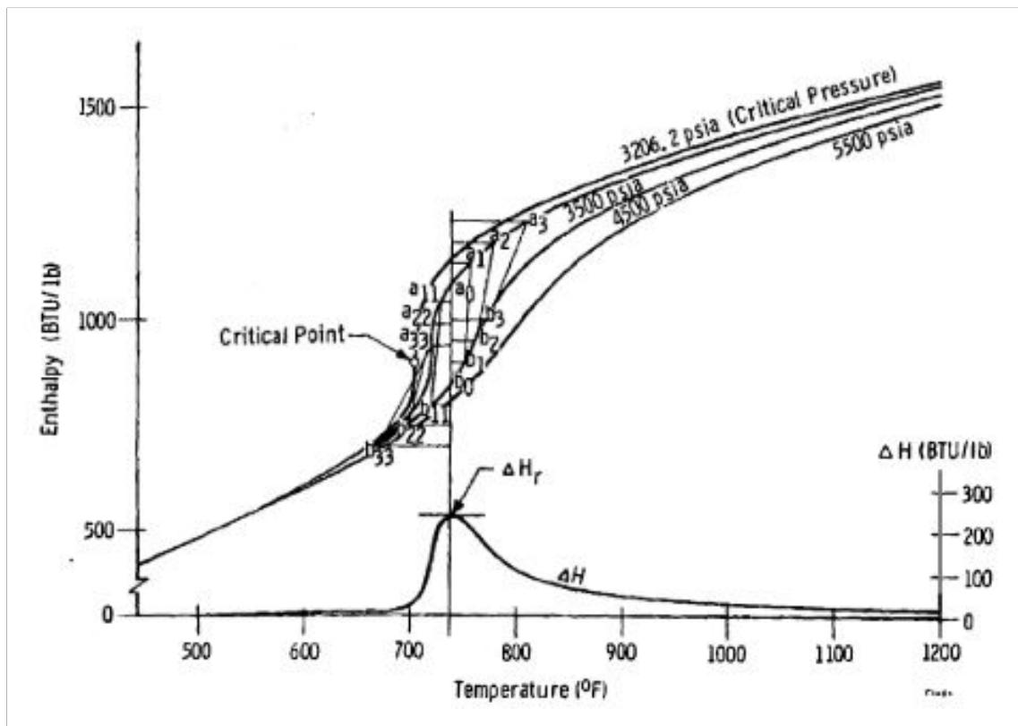
Figure 5.4: Enthalpy-Temperature diagram of  $\text{CO}_2$  illustrating the Pinch-point problem. Source: Feher [1968]
