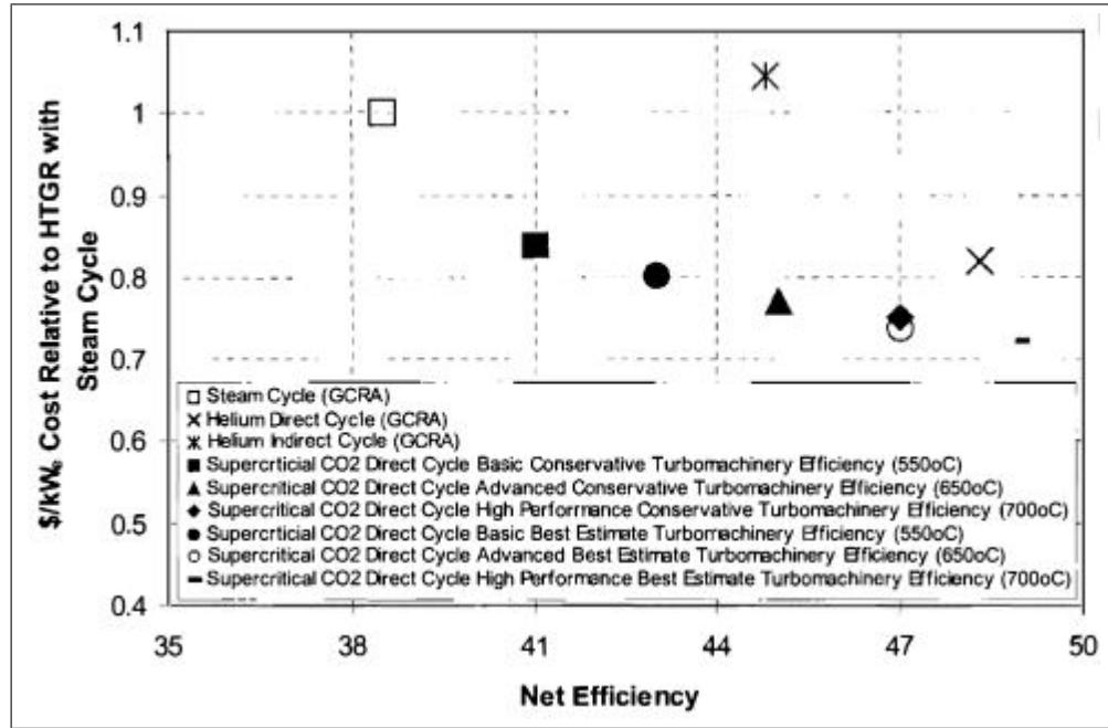
Figure 5.6: Net efficiency and relative costs for different power cycles (\$/kW<sub>e</sub>). Source: Dostal [2004]
