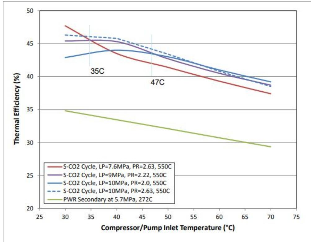
Figure 5.9:  $sCO_2$  power cycle efficiency at  $550^\circ C$  with increasing compressor inlet conditions.
