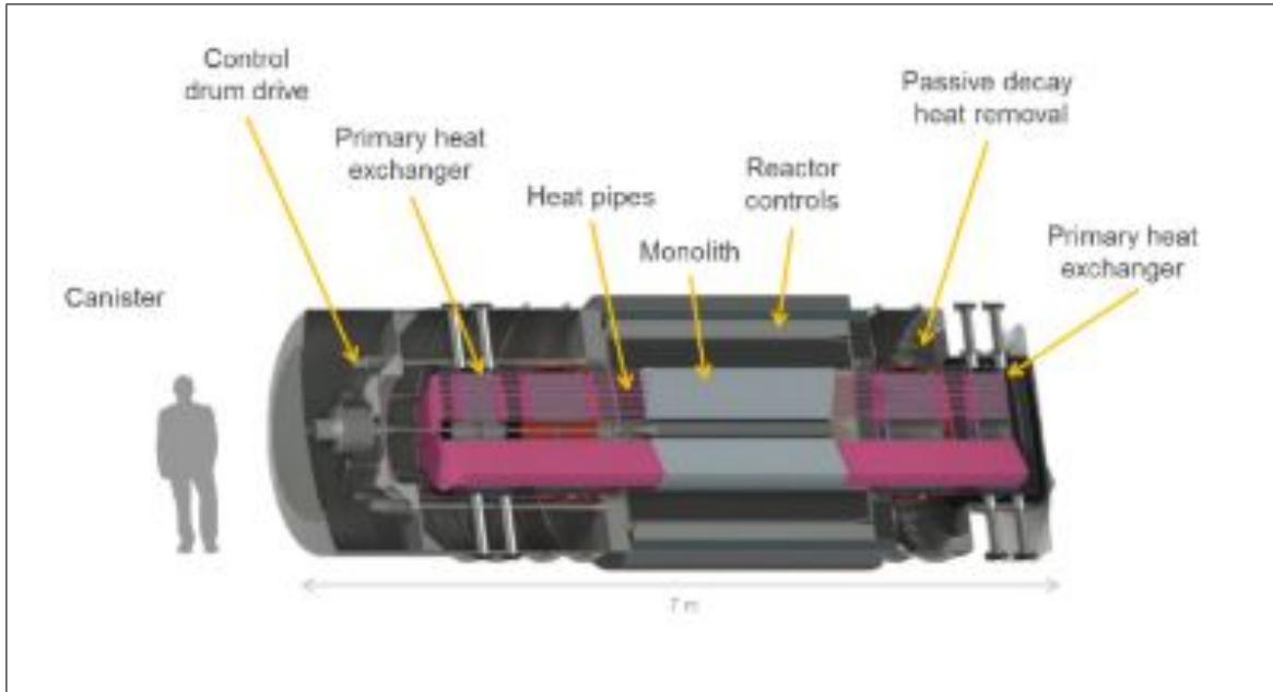
Figure 4.1: eVinci Reactor System Overview. Source: Levinsky et al. [2018]
