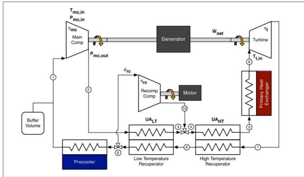
Figure 5.8: Recompression cycle diagram. Source: Dyreby [2014]
