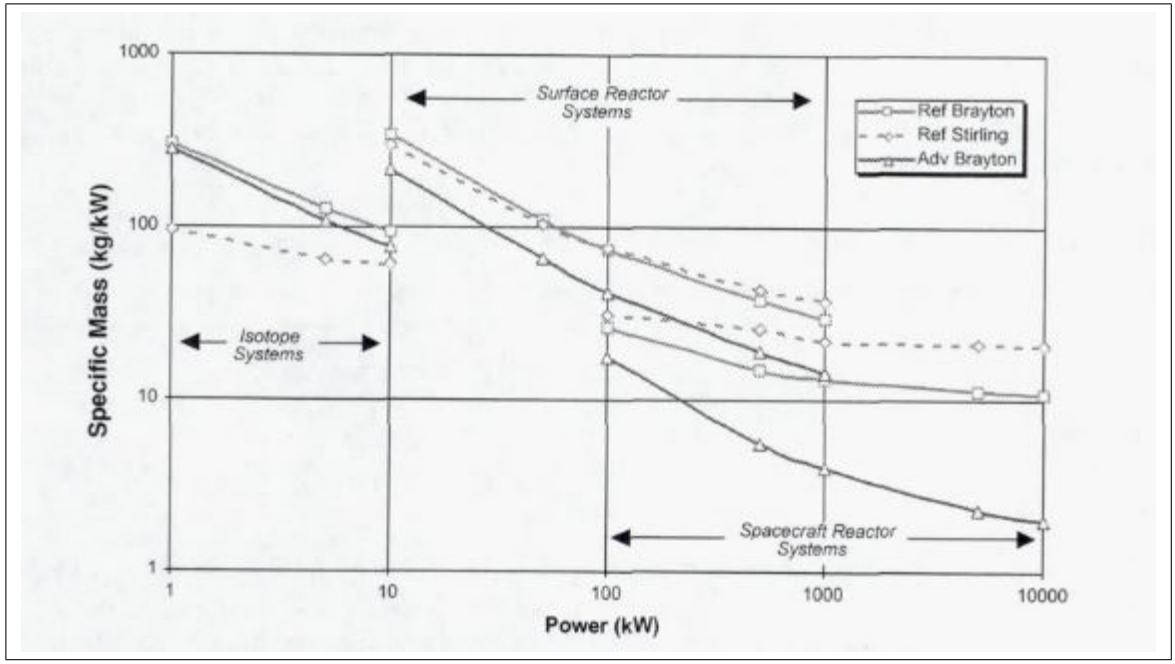
Figure 5.3: Summary of Specific Mass Projections for Brayton and Stirling Power Systems.
