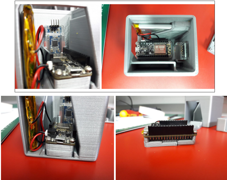
Figure C.1: Electronic core inside the internal support structure of the first ball.
