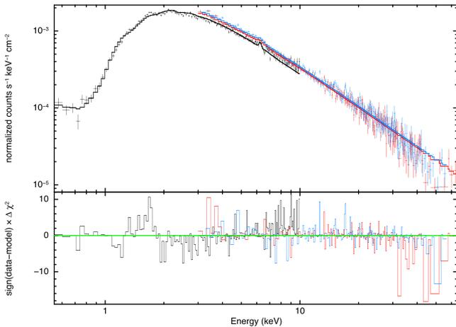
**Figure 3.** Data, fit model (top panel) and residuals (bottom panel) for *XMM-Newton* (black) and *NuSTAR* FPMA (red) and FPMB (in blue) spectra when the parameters are all tied to the best-fitting parameters from the *XMM-Newton* spectral fit.
