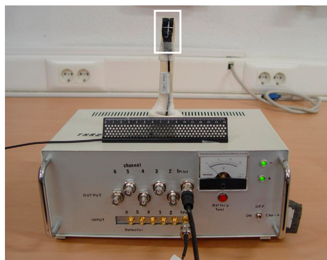
Fig. 1. One of the TNRD detectors (marked with a white box) and associated six electronics channels.
