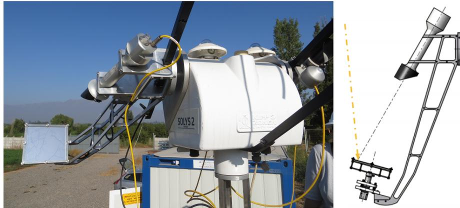
Figure 2-3: Left: TraCS mounted to a Sun Tracker on a sun tracker in San Felipe, the mirror mounted to the plate is the reference glass mirror. Right: TraCS setup with the pyrheliometer facing the mirror (CSP Services, 2016).
