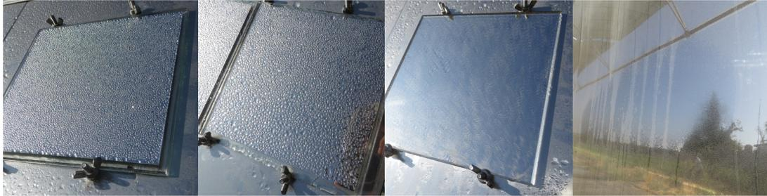
Figure 2-5: Pictures of samples and the collector on the 8th of March at 9.30 hrs. From left to right: anodized aluminum films, polymeric films, glass mirror and the actual parabolic trough collector.
