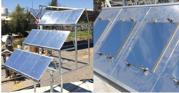
Figure 2-2: Stand-alone structure installed in San Felipe. Left: Structure with the aluminum sheets with its screws for installing the mirror samples. Right: Mirror samples installed on the aluminum sheets.
