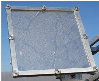
Figure 2-10: Reference mirror on the 15th of March. Non-uniform soiling can be noticed with traces of drop of water rolling down the surface.
