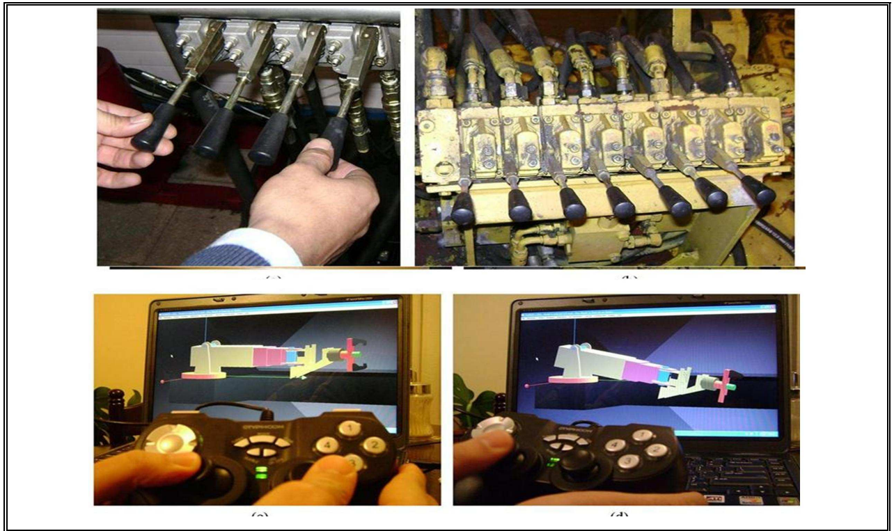
FIGURE 3.12. Real and Mockup Manifold for the manipulator (above). Conventional joystick control (below).
