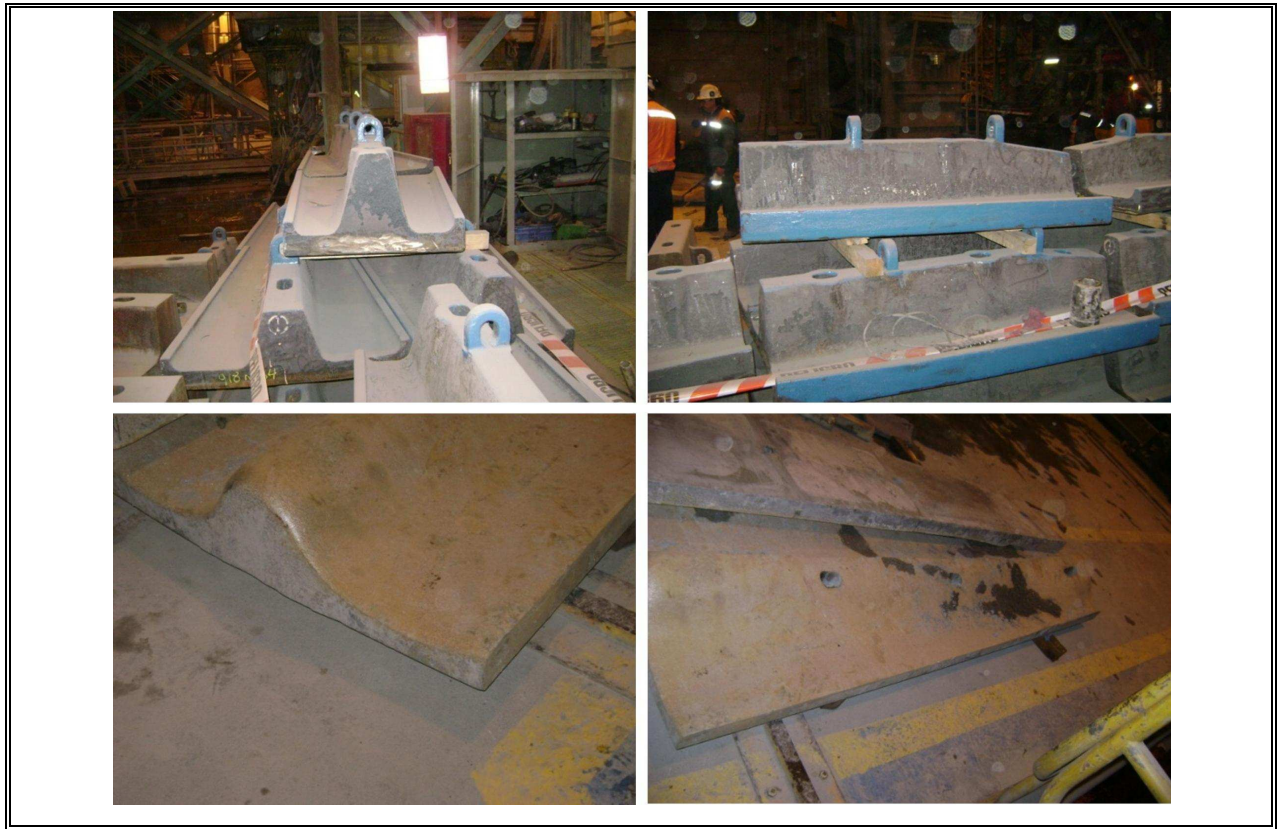
FIGURE 3.3. New Liners (above). Liners with wear (below).
