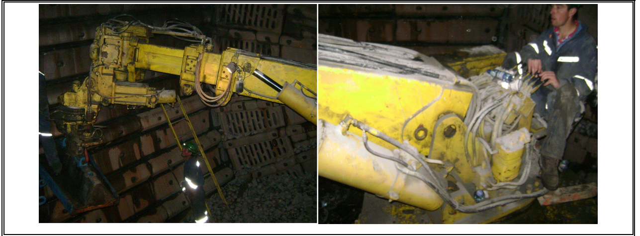
FIGURE 3.4. Real Liner Manipulator.
