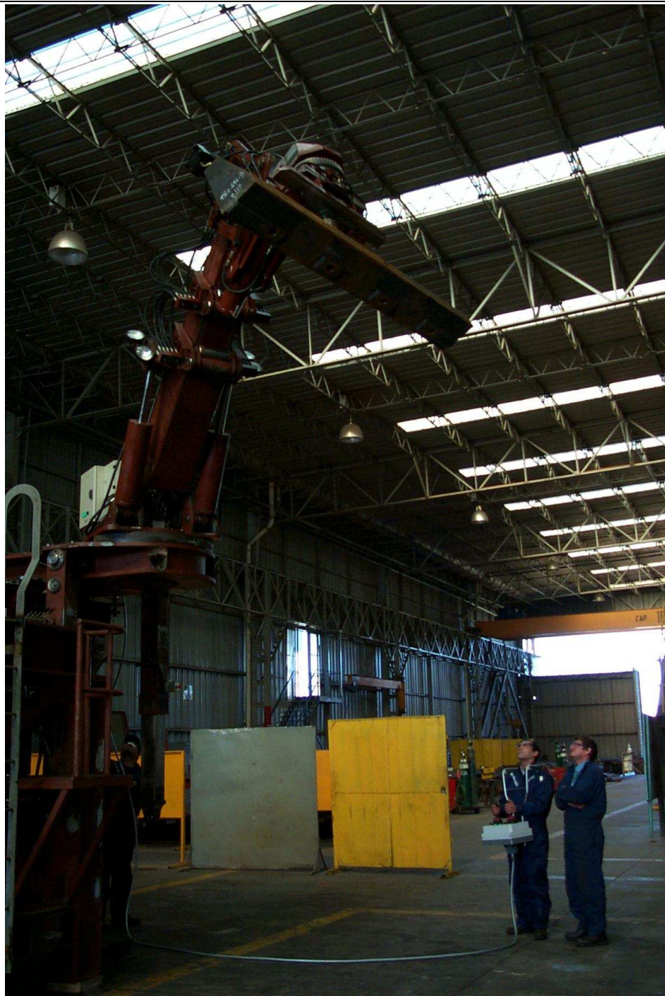
FIGURE 3.11. Manipulator operated with a wired control.
