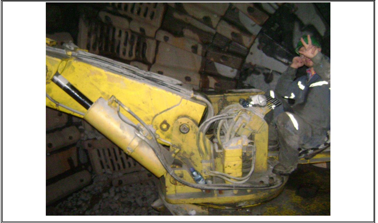
FIGURE 3.6. Operator at the command of the manipulator of liners.
