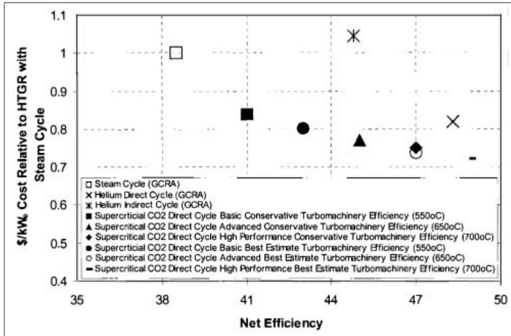
Figure 5.6: Net efficiency and relative costs for different power cycles ( $\$/kW_e$ ). Source: Dostal [2004]
