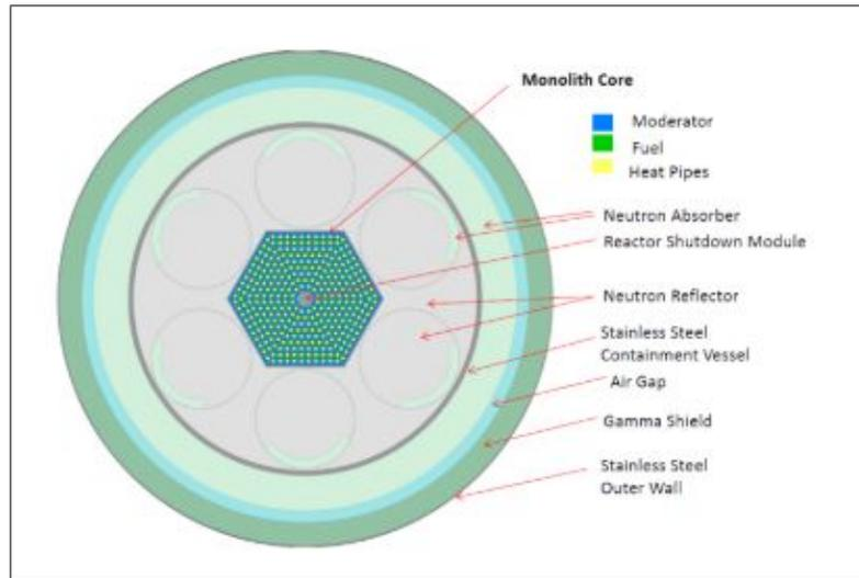
Figure 4.2: eVinci reactor cross section, showing the core and surrounding structures. Source: Levinsky et al. [2018]
