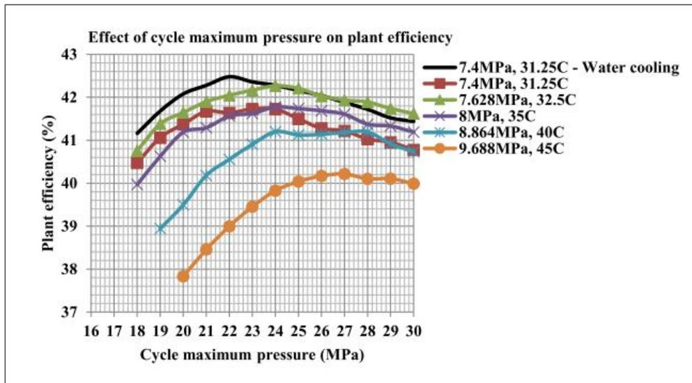
Figure 5.10: Effect of cycle maximum pressure on plant efficiency. Source: Moisseytsev et al. [2016]
