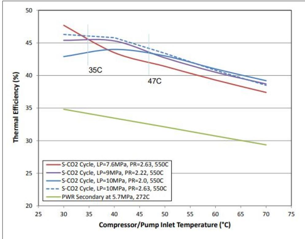
Figure 5.9:  $sCO_2$  power cycle efficiency at  $550^\circ C$  with increasing compressor inlet conditions. Source: Conboy et al. [2015]
