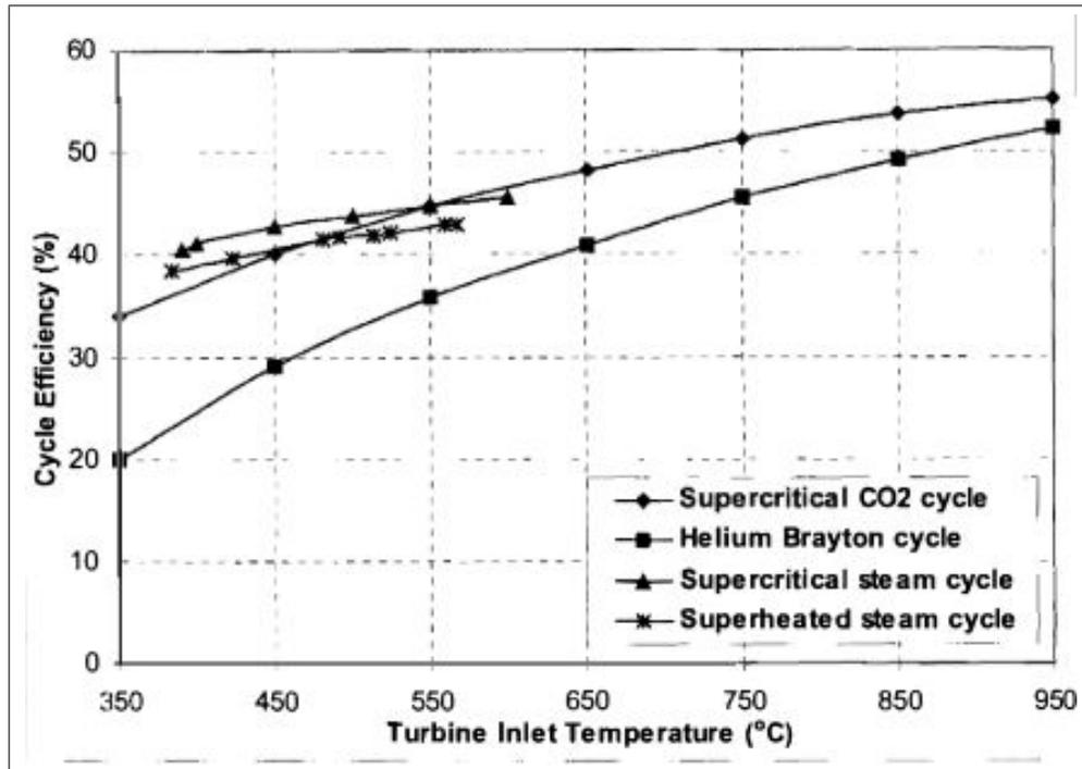
Figure 5.7: Cycle efficiency comparison of advanced power cycles. Source: Dostal [2004]
