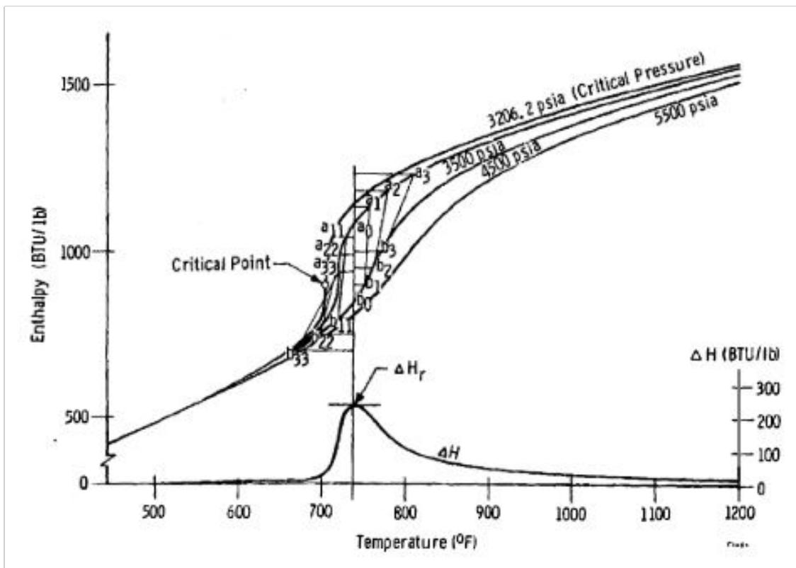
Figure 5.4: Enthalpy-Temperature diagram of  $CO_2$  illustrating the Pinch-point problem. Source: Feher [1968]
