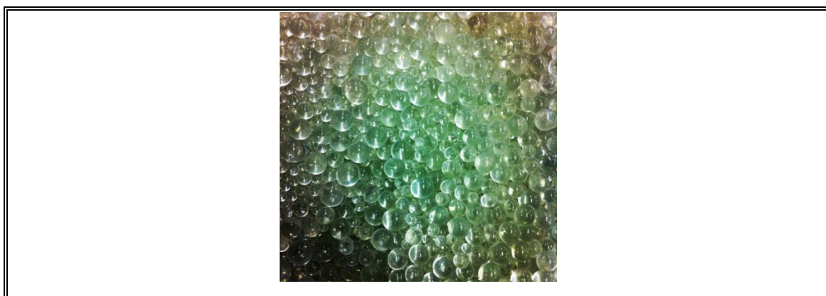
Figure 4.2: Synthetic material made of glass beads
