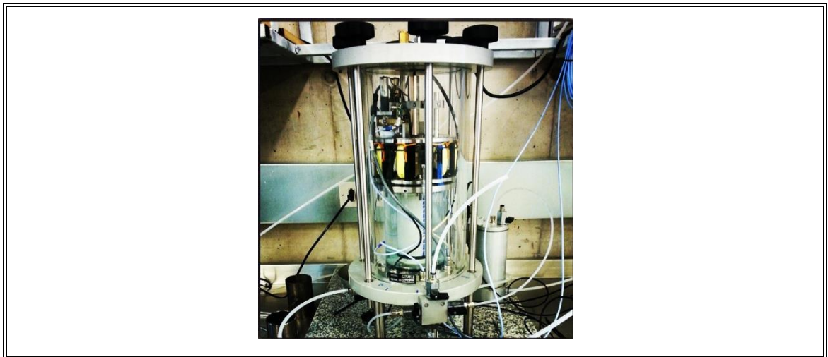
Figure 2.3: CONTROLS® device used to conduct TS tests
