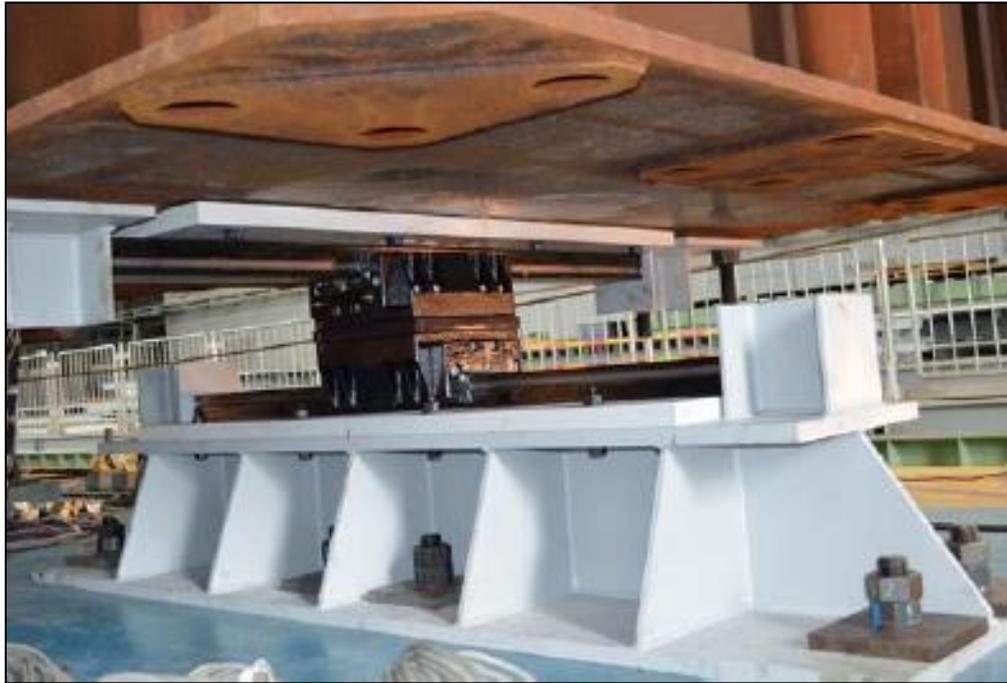
Figure 1.3. Photo of installed CL bearing illustrating orthogonal LM guides assemblies on top and bottom (Ryan et al, 2013).
