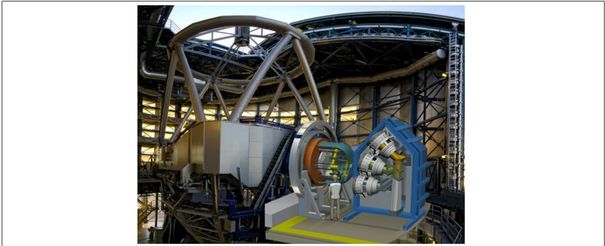
Figure 1.1. MOONS instrument mounted on the telescope. The spectrograph is in the left, the front-end in the centre and one of the VLT's on the right (Cirasuolo et al., 2014).
