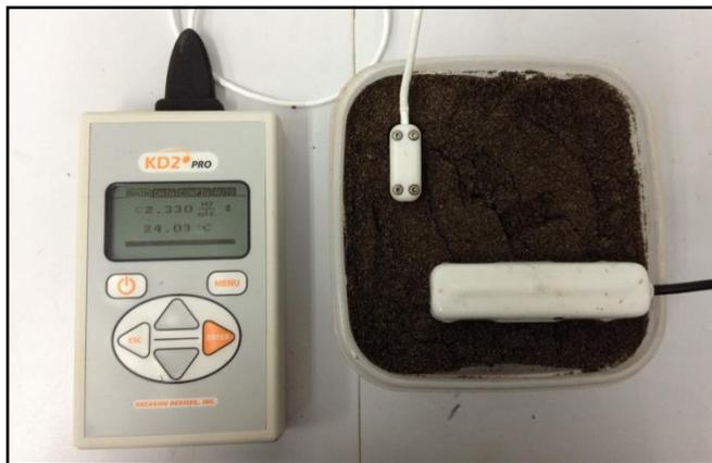
Figure 3-3: Experimental setup to determine the thermal properties as a function of soil water content.
