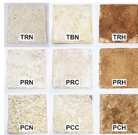
**Figura 7.** Tabla de materiales probados en el estudio. Appels, F., Karana, E., Jansen K.M.B., Camere, S., Montalti, M., Dijksterhuis, J., . . . H.A.B. (2019). Fabrication factors influencing mechanical, moisture- and water-related properties of mycelium-based composites. *Materials & Design*, 161, 64-71.
