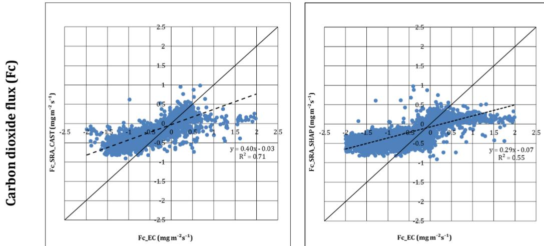
**Figure 1.** Comparison between sensible heat ( $H$ ), latent heat ( $\lambda E$ ) and dioxide carbon fluxes ( $F_c$ ) estimation from surface renewal analysis (SRA) using Castellvi method (Cast) and Shapland method (Shap) against eddy covariance (EC). Data was pooled to represent all stability conditions.
