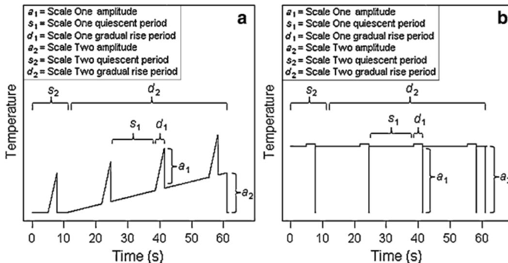
Fig. 4 Ramp models of the Shapland procedure. a) The traces of a two-scale ramp model. b) the first-order structural function of a two-scale ramp model. Extracted from Shapland et al. (2012a).
