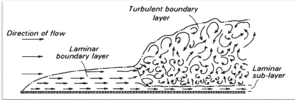
Fig. 1 Eddies of different sizes develop in the turbulent boundary layer. The laminar boundary layer develops over a flat surface and subsequently transitions to turbulent flux. Extracted from Oke (1990).
