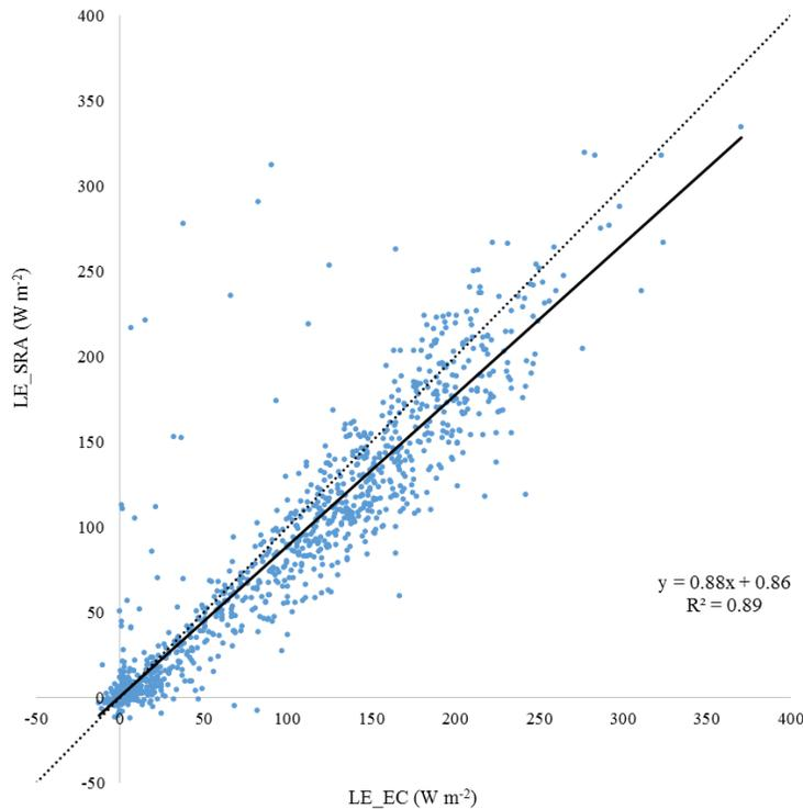
Fig. 3 Comparison between latent heat flux ( $LE$ ) estimated by eddy covariance ( $LE_{EC}$ ) and surface renewal analysis ( $LE_{SRA}$ ), for all stability conditions. The solid lines represents the linear regression analysis and the dotted line the 1:1 relationship.
