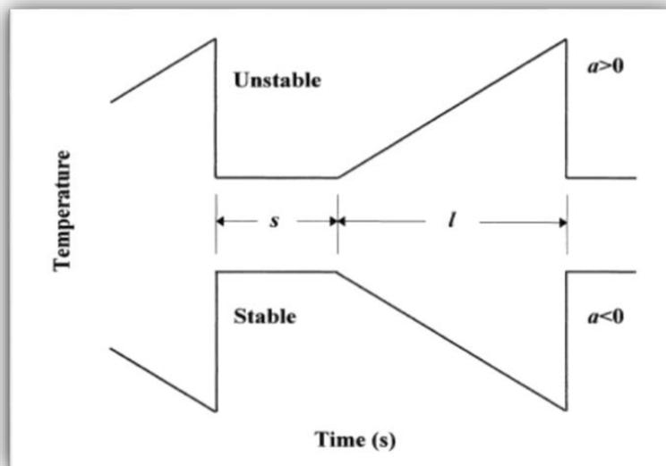
Fig. 3: Ramp model in stable and unstable atmospheric conditions, extracted from Spano et al. (2000).
