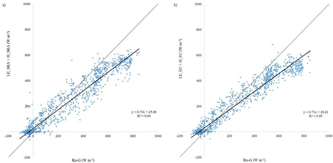
Fig. 6 Energy balance closure for surface renewal analysis (a) and eddy covariance (b) for January 2018 in a vertically trellised vineyard for all stability conditions. The solid lines represent the linear regression analysis and dotted lines the 1:1 relationship.
