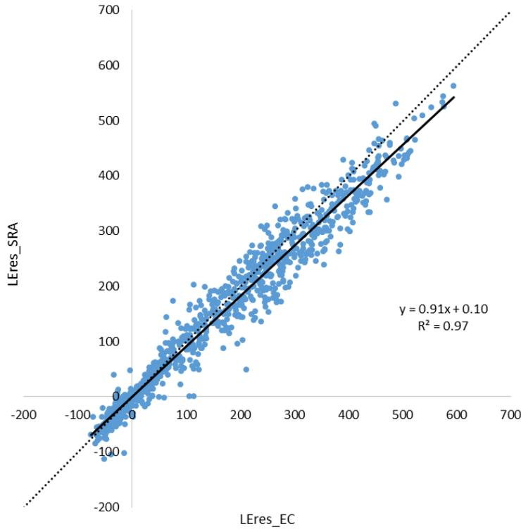
Fig. 5: Comparison between latent heat flux estimated as residual from energy balance equation by eddy covariance (LEres\_EC) and surface renewal analysis (LEres\_SRA), for all stability conditions. The solid line represents the linear regression analysis and dotted line the 1:1 relationship.
