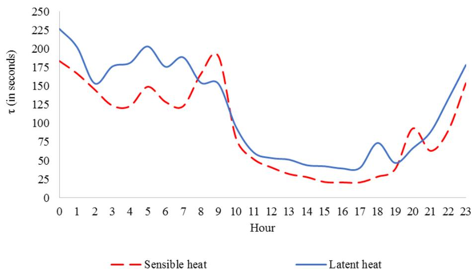
Fig. 7. Averages of the 30 min values for ramp duration ( $\tau$ ) by hour for latent heat (solid line) and sensible heat (dotted line) fluxes for January 2018.
