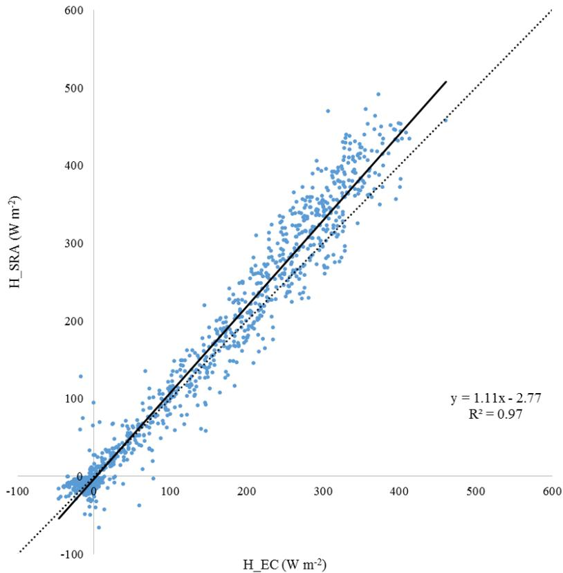
Fig. 2 Comparison between sensible heat flux ( $H$ ) estimated by eddy covariance ( $H_{EC}$ ) and surface renewal analysis ( $H_{SRA}$ ) for all stability conditions. The solid line indicates the linear regression analysis and dotted line the 1:1 relationship.
