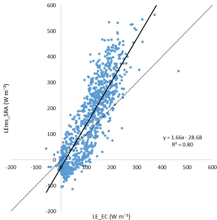
Fig. 4 Comparison between latent heat flux (LE) estimated by eddy covariance ( $LE_{EC}$ ) and by surface renewal analysis as residual from energy balance equation ( $LE_{res\_SRA}$ ), for all stability conditions. The solid line represents the linear regression analysis and dotted line the 1:1 relationship.
