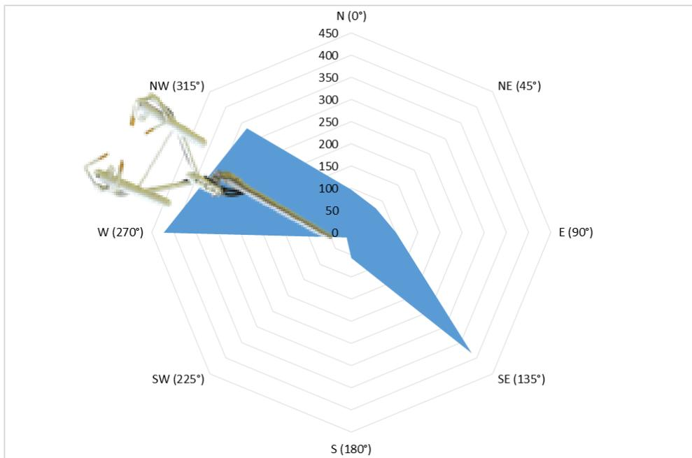
Fig.1. Top: Footprint generated using data gathered in unstable atmospheric conditions using Kljun et al. (2015). IRGASON real orientation (azimuth 270°). Bottom: Wind rose for January 2018 using all atmospheric conditions, numbers indicate number of events from that direction.
