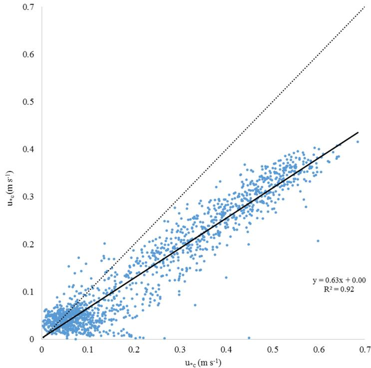
Fig. 8 Friction velocity measured with IRGASON ( $u_{*c}$ ) vs estimates by equation (10) ( $u_{*c}$ ). The solid line represents the linear regression analysis and the dotted line the 1:1 relationship.
