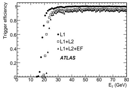
**Figure 4.** L1, L2 and EF efficiencies of e22i trigger item for single electrons as function of electron  $p_T$ .
