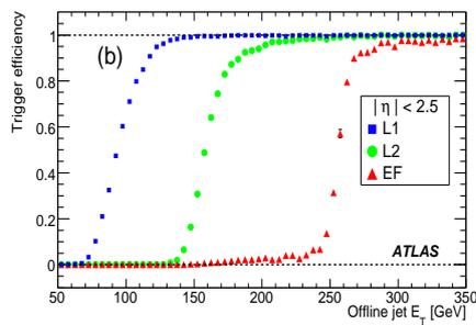
**Figure 6.** L1, L2 and EF efficiency of jet255 item as function of the offline jet transverse energy. The thresholds applied are 70/150/255 GeV for L1/L2/EF, respectively.
