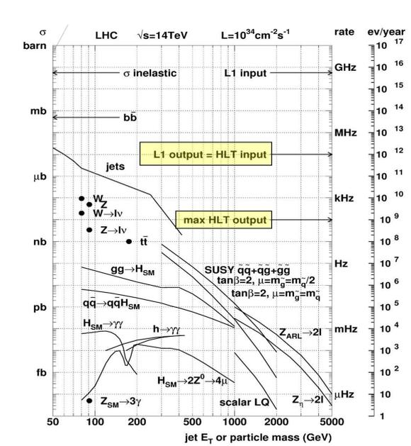
**Figure 1.** The expected cross-section (left axis) and corresponding event rate at  $10^{34}\text{cm}^{-2}\text{s}^{-1}$  instant luminosity for different processes. Also shown L1 and HLT output rates.
