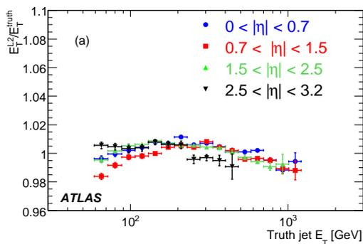
**Figure 2.** Jet energy scale for the L2 jets as a function of the truth jet  $E_T$  for four different bins in  $\eta$ .
