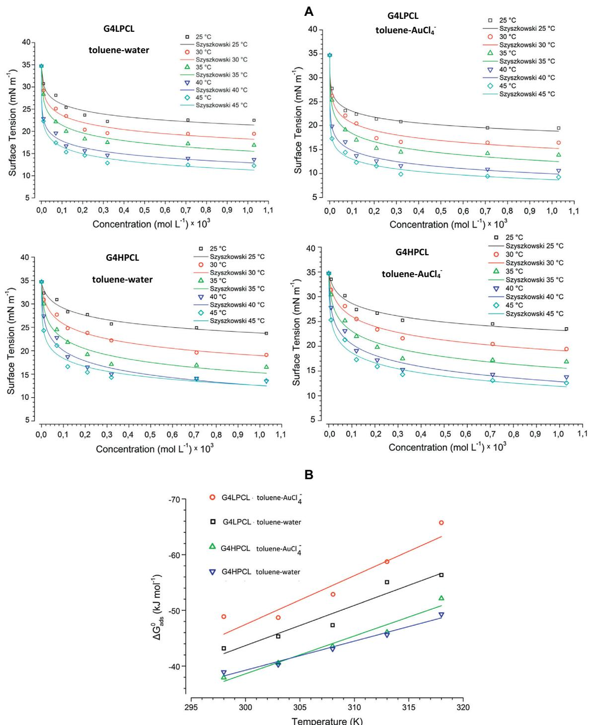
**Fig. 1.** (a) Interfacial tension as a function of PAMAM-PCL concentration at the respective interfaces and at different temperatures. (b) Standard free energies of adsorption as a function of temperature for G4LPCL and G4HPCL for each interface.
