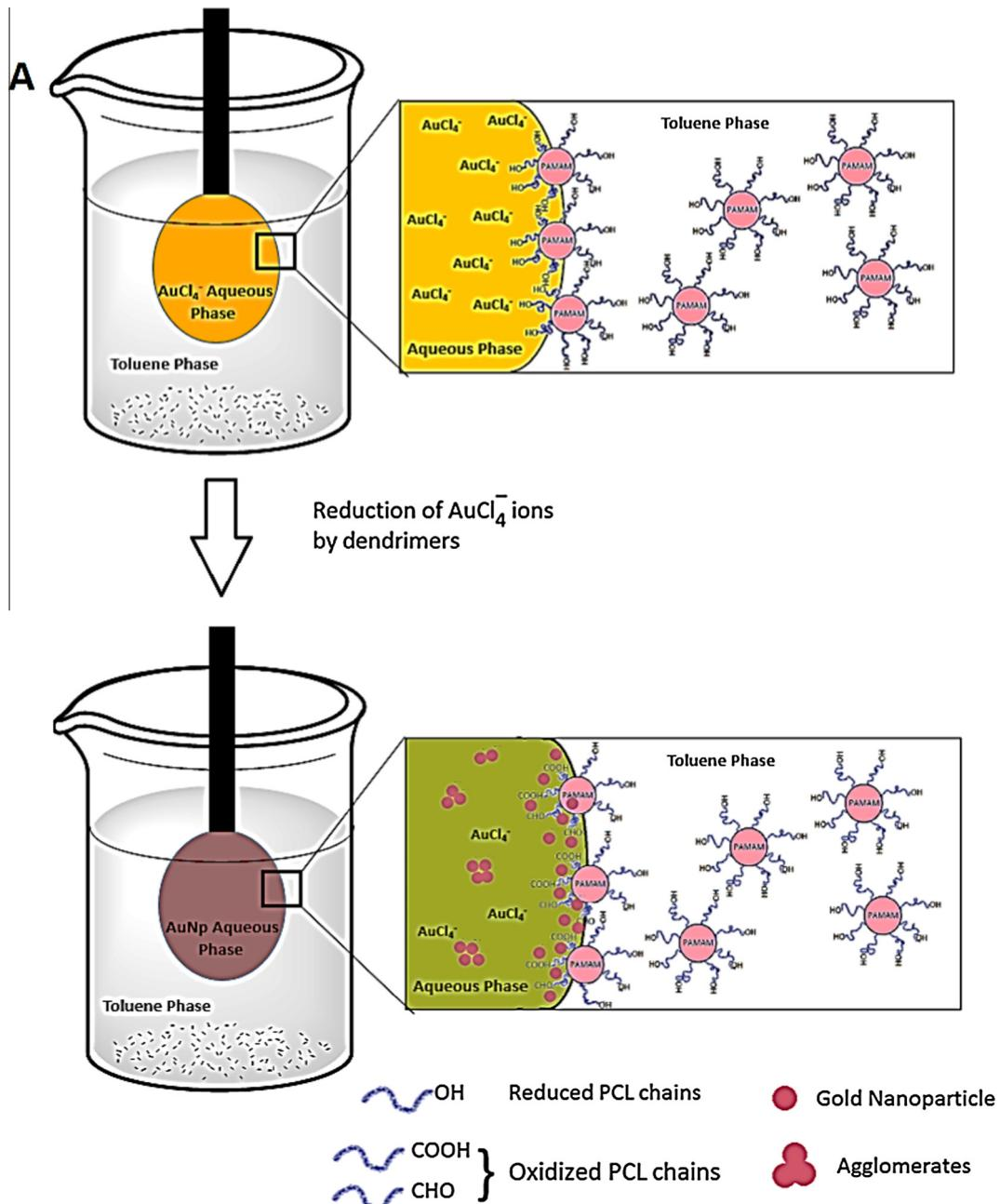
**Scheme 1.** Illustration of the synthesis of gold nanoparticles with PAMAM-PCL dendrimers at the (a) toluene- $\text{AuCl}_4^-$  solution and (b) air- $\text{AuCl}_4^-$  solution interfaces.
