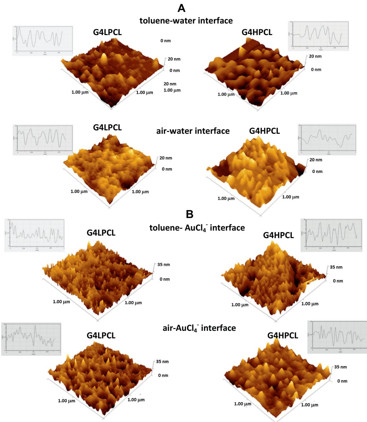
**Fig. 3.** AFM images obtained for GL4PCL and G4HPCL dendrimers and the respective obtained gold nanoparticles at the (a) toluene-water and air-water interfaces and at the (b) toluene- $\text{AuCl}_4^-$  and air- $\text{AuCl}_4^-$  interfaces. The topographies of dendrimers and gold nanoparticles correspond to 1 h after deposition of monolayers at 298 K. The insets correspond to surface-roughness profiles for each sample.
