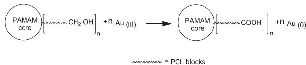
According to this mechanism, the redox reaction could produce the oxidized form of a hydroxyl end group (i.e., a carboxylic acid group) and metal atoms. In addition, a schematic representation of these reactions and possible interactions as well as further formation of gold nanoparticles at both interfaces is depicted in [Scheme 1](#).
