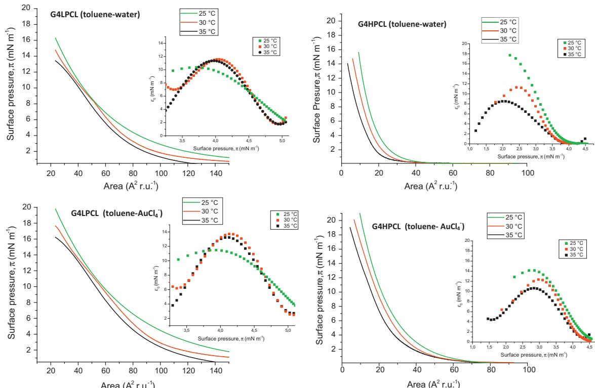
**Fig. 2.** Surface pressure–area isotherms for PAMAM-PCL dendrimers at different temperatures for each interface. The insets correspond to the static elasticity modulus as a function of the surface pressure.
