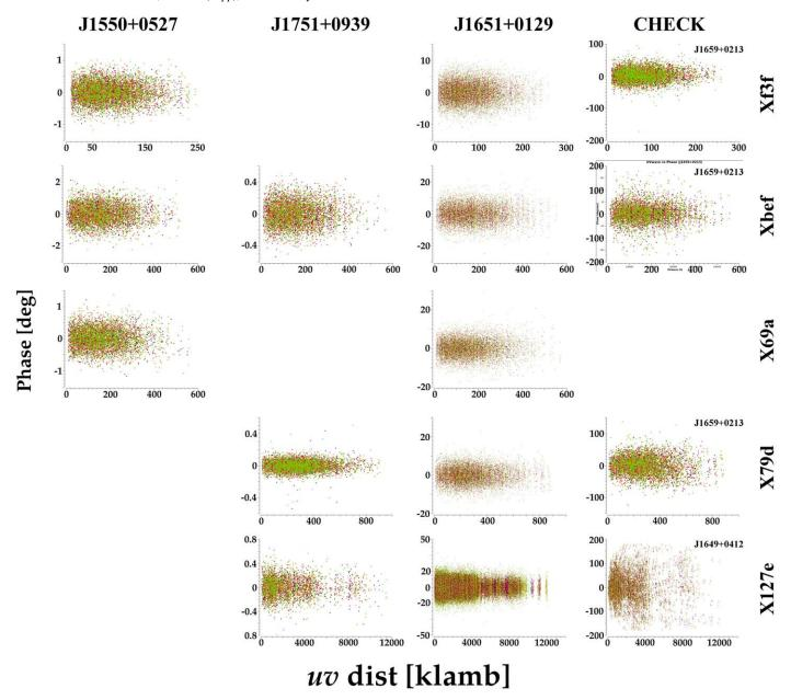
Figure 13. Phase vs. uvdistance visibility distributions obtained after the WVR solution scaling for the pointlike sources used as calibrators in the observations considered in this work.
