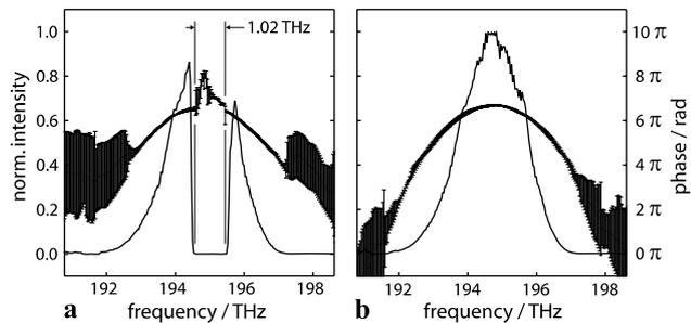
**Fig. 6** Measured spectral intensity and retrieved phase of the signal. Averages of five independent measurements each. (a) Mask applied. There is a 1 THz spectral gap. (b) Mask removed for comparison
