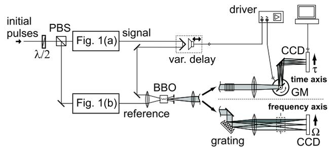
**Fig. 3** Schematic of the experimental arrangement. PBS: polarizing beam splitter, BBO: non-linear crystal, GM: galvanometer scanner. The BBO crystal generates the cross-correlation of signal and reference, and a diffraction grating disperses it. The spectra are focused on an electronic camera (CCD) to obtain the VAMPIRE spectrogram. The delay axis is swept by a mirror mounted on a galvanometer scanner actuated synchronously with the variable delay of the signal
