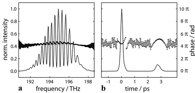
**Fig. 5** Spectral (a) and temporal (b) intensity and phase of the reference pulse obtained from 10 independent measurements. The double pulse structure (b) with different chirp and peak power is evident. The pulse separation is  $\approx 2.8$  ps
