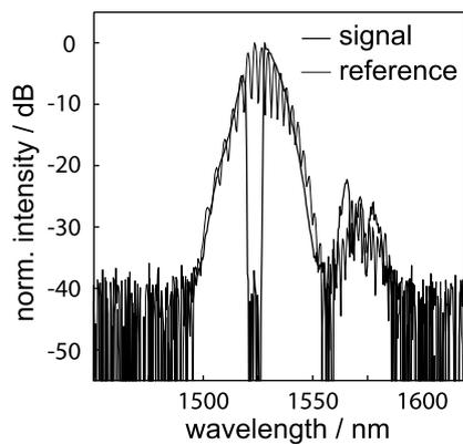
**Fig. 2** Spectra of signal, with the cut spectral region, and reference pulse, which covers the spectral region of the signal
