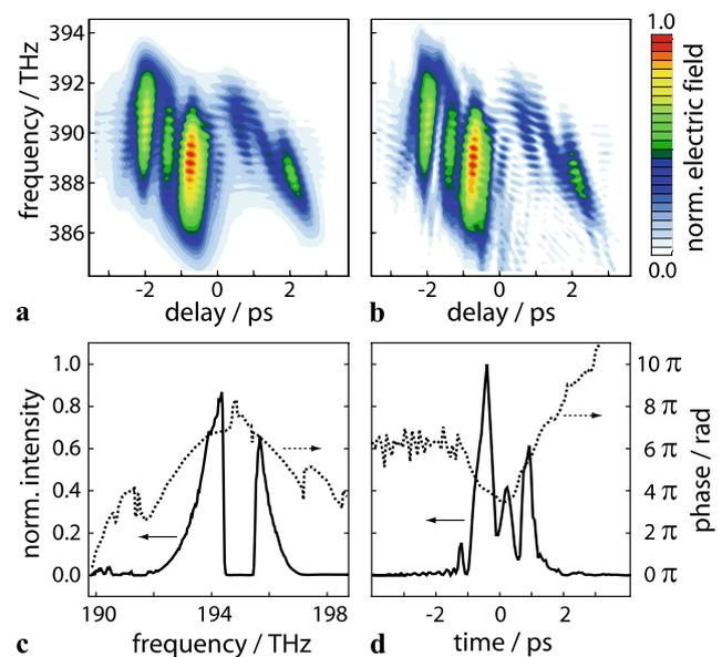
**Fig. 4** Measured (a) and reconstructed (b) VAMPIRE spectrogram (electric field amplitude). (c) Independently measured spectrum and reconstructed spectral phase function of the signal. (d) Temporal pulse shape and phase function of the signal as obtained from a Fourier transform of (c)
