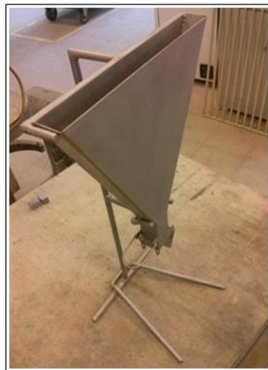
Figure 8-2: Mortar V-funnel Test
