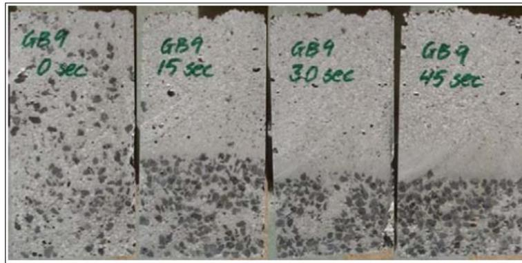
Figure 2-4: Cylinders samples vibrated for 0, 15, 30 and 45 seconds. (Mackechnie et al., 2007)
