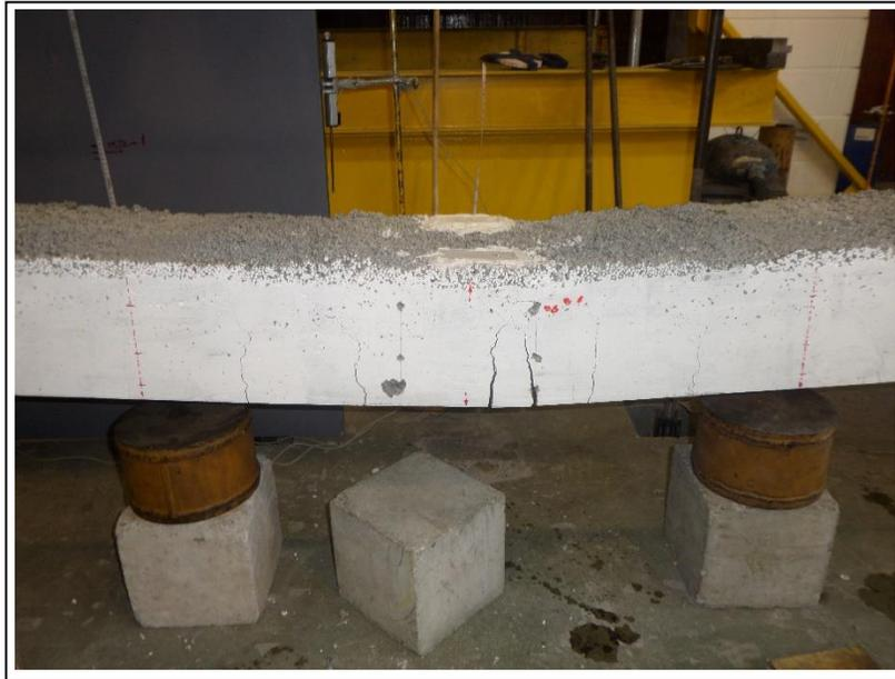
Figure 6-8: Typical crack pattern and failure mode of flexural tests.
