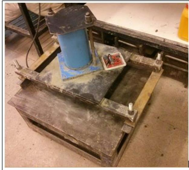
Figure 8-1: Vibratory table and accelerometer
