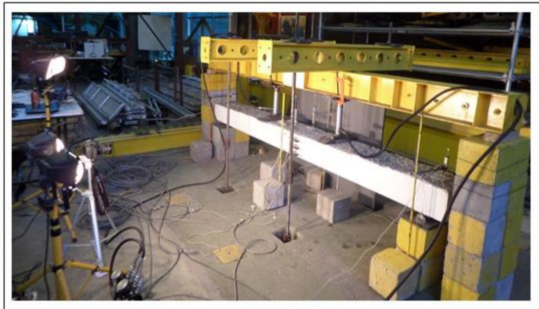
Figure 8-5: Monotonic load test set up
