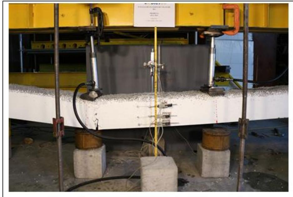
Figure 8-10: Failure mode SCS-1 specimen
