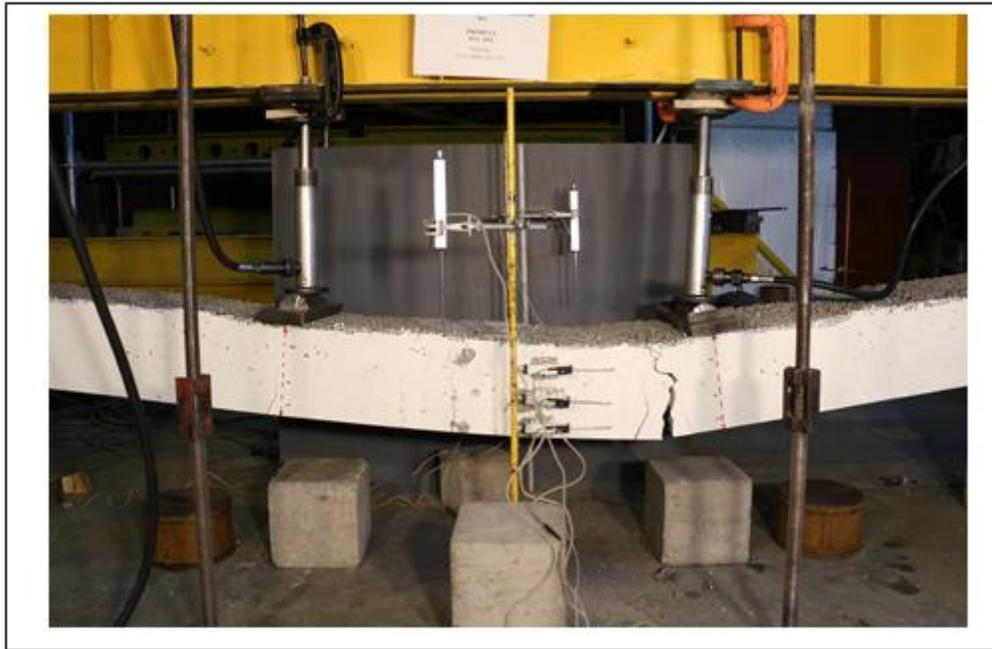
Figure 8-6: Failure mode SCG-1 specimen
