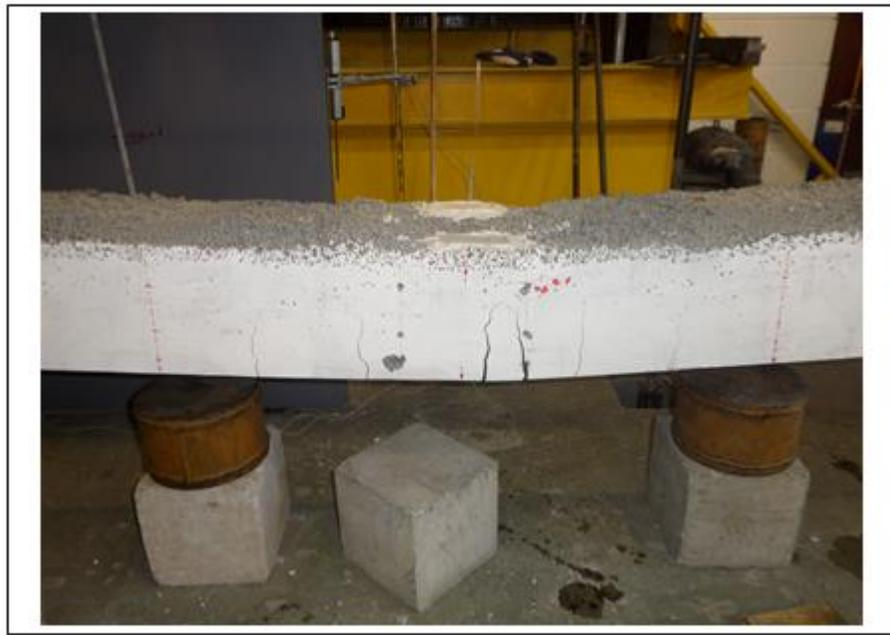
Figure 8-12: Failure mode SCS-1 specimen
