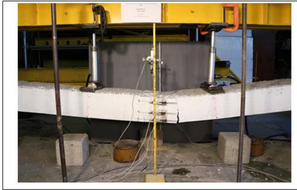
Figure 8-8: Failure mode SCG-2 specimen
