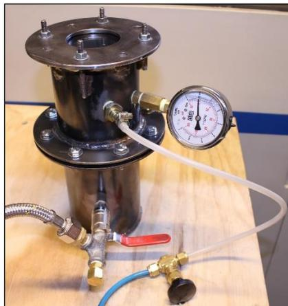
Figure 2-2: Chamber used to fabricate the specimens.
