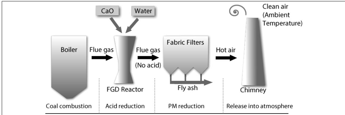
Figure 1.1. Power plant diagram with fabric filters collection system
