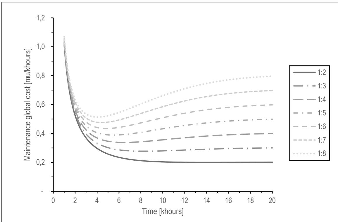
Figure 6.2. Replacement interval sensitivity analysis for different cost ratios ( $C_p : C_c$ )
