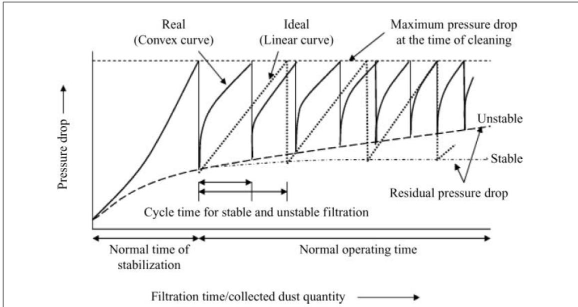
Figure 1.4. Performance curve for filters in a multiple compartment [Mukhopadhyay, 2009]
