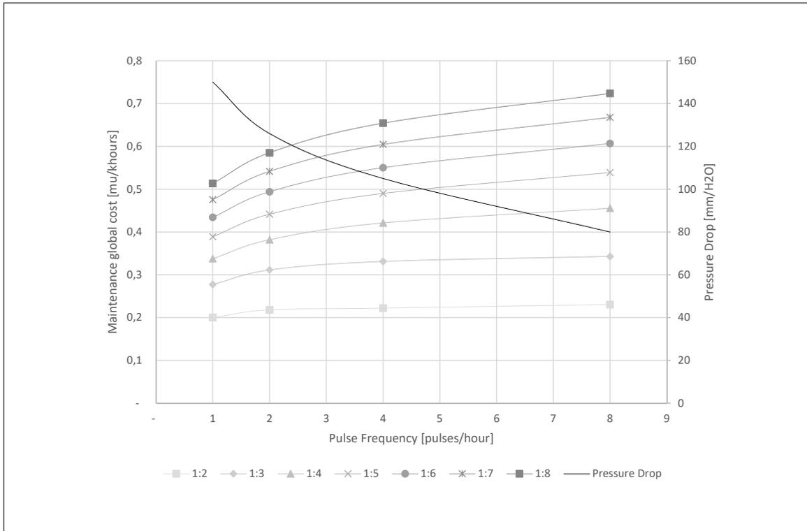
Figure 5.4. Optimal pulse frequency with different costs ratios
