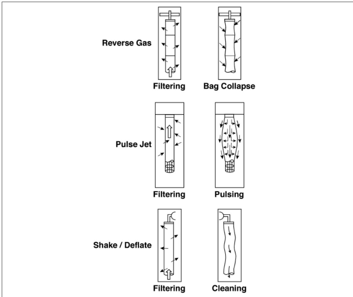
Figure 1.2. Fabric filters cleaning methods [Miller, 2015]
