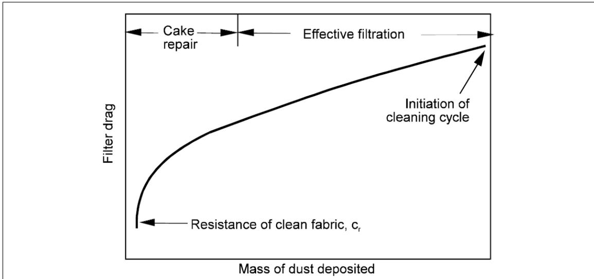
Figure 1.3. Performance curve for a single woven bag [Beachler et al., 1995]
