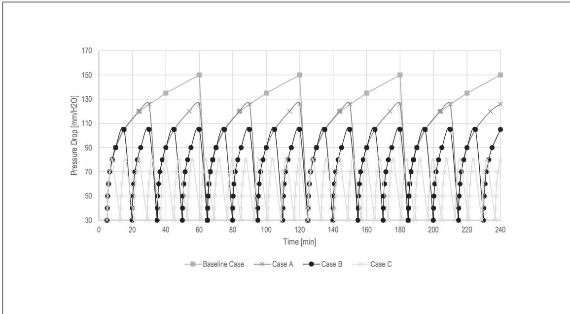
Figure 4.1. Pressure drop in time with different pulses frequencies
