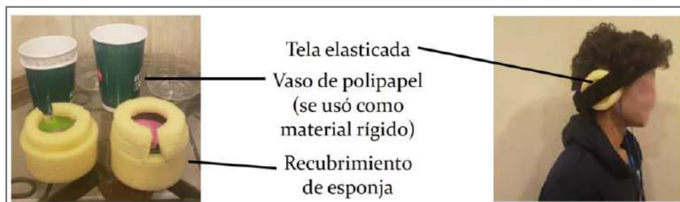
Figure 4-A.3: Example of the home-made mock-up presented as part of the Final Team Presentation to Stakeholders, Team 28. Soundblock; in the mock-up the materials are identified: stretch fabric (tela elasticada), polypaper cup used as rigid material (vaso de polipapel, se usó como material rígido), and sponge coating (recubrimiento de esponja).
