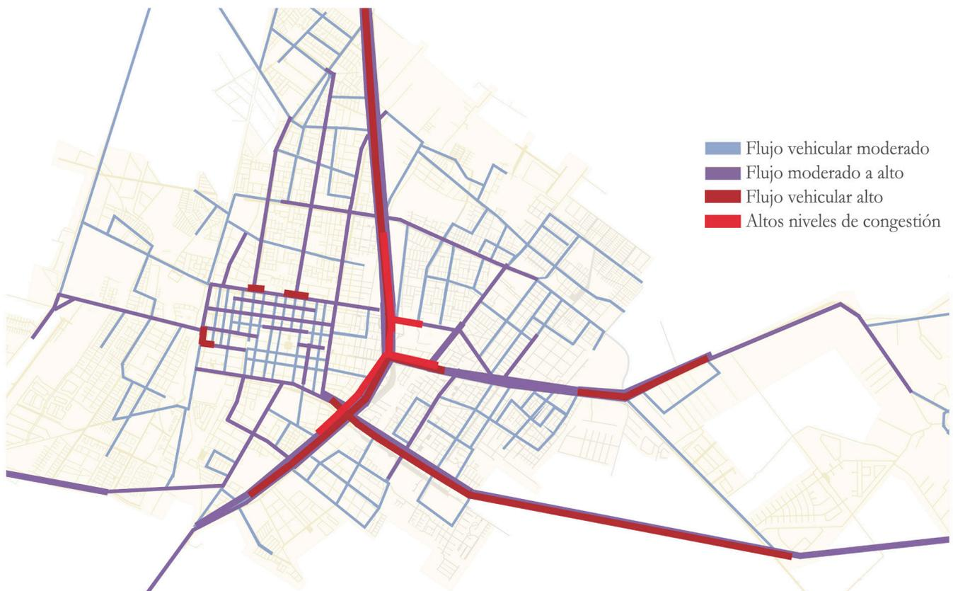
Fig (8): CARGA VEHICULAR DE LA RED VIAL
