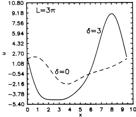
FIG. 2. Solution for  $u(x,t)$  obtained from the integration of the three-mode system, after reaching the fixed point. For  $\delta=0$  the solution is steady; for  $\delta=3$  it is traveling to the left with speed 0.199.
