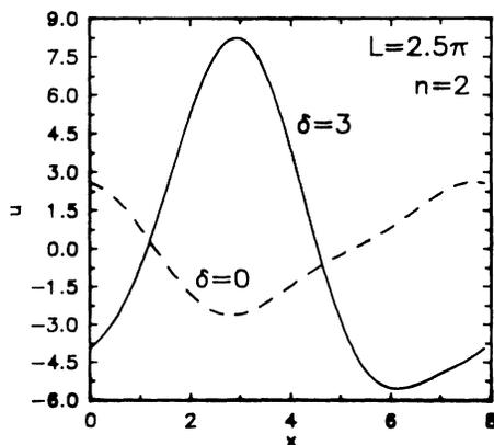
FIG. 1. Wave form  $u(x,t)$  obtained from a numerical integration of the two-mode system, shown once the fixed point is reached. In all figures the dotted line shows the final state for  $\delta=0$ . For  $\delta=0$  the solution is steady; for  $\delta=3$  it travels to the left with speed 1.169.
