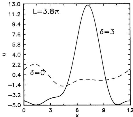
FIG. 3. Solution for  $u(x,t)$  for a different value of  $L$  obtained from the integration of the three-mode system, after reaching the fixed point. Now for  $\delta=0$  the solution may travel to the right or the left with speed 0.369. For  $\delta=3$  it travels to the right with speed 1.516.
