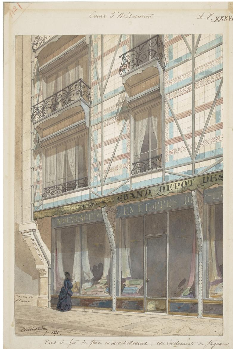
**Fig. 04** “House with iron structure with glazed earthenware cladding” Eugène Emmanuel Viollet-le-Duc, 1871.
