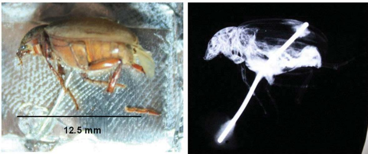
Figure 7: Insect radiography using Tungsten X-pinch of 7.5 μm.
