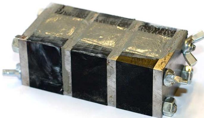
**Figure B.1** 3-gang 20mm side mold for RCM-based pastes
