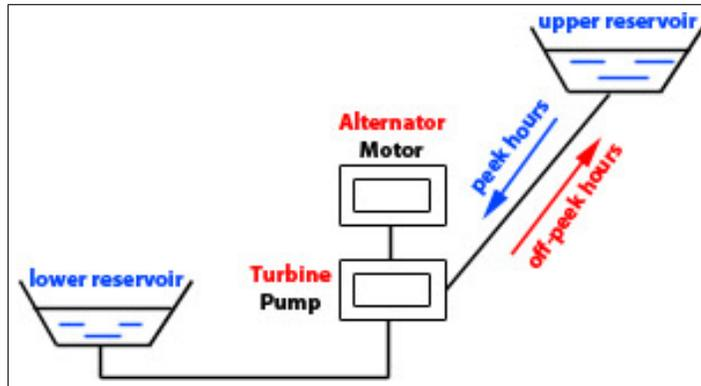
FIGURE 5.1. Pumped Hydro Storage System
