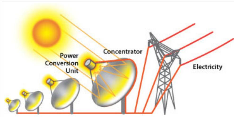
FIGURE 3.6. Stirling Solar Dish Energy Conversion Process (US DOE, 2010)
