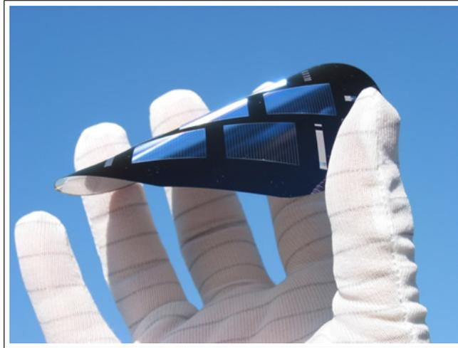
FIGURE 3.7. Thin-Film PV Panel (NREL, 2008)
