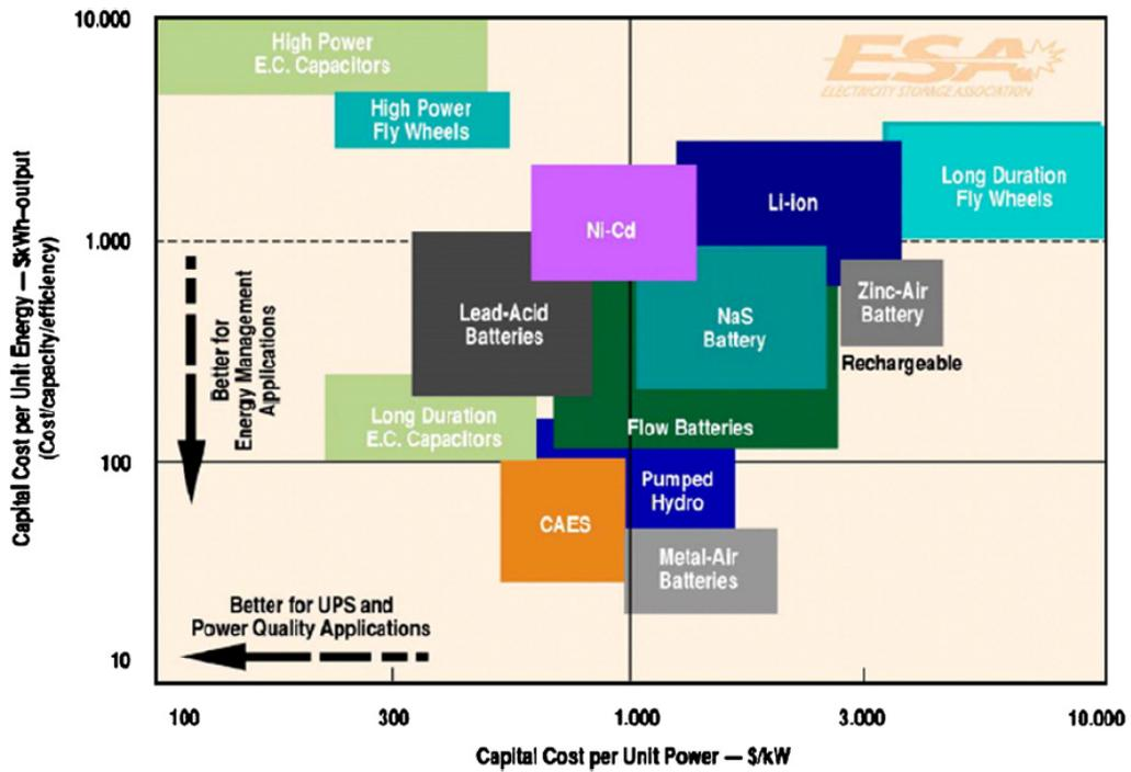
FIGURE 5.11. Investment Costs per Unit and Power or Unit of Energy for Different Storage Technologies (Ibrahim et al., 2008)
