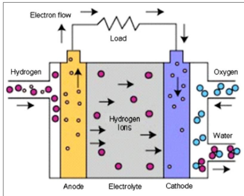
FIGURE 5.5. Fuel Cells-Hydrogen Energy Storage (Ibrahim et al., 2008)
