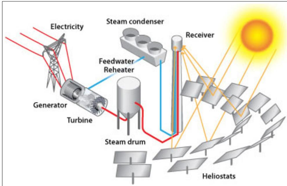
FIGURE 3.3. Solar Power Tower Energy Conversion Process (US DOE, 2010)
