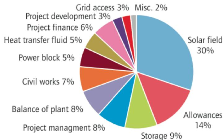
FIGURE 4.1. Percentages of investment cost of a 50MW trough plant with 7-hour storage (IEA, 2010a)
