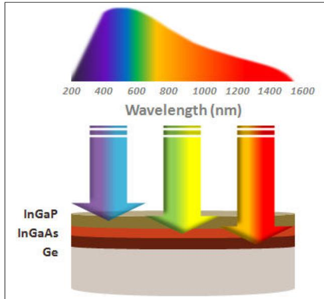
FIGURE 3.8. Multi-junction Cell Spectrum Absorption (US DOE, 2010)
