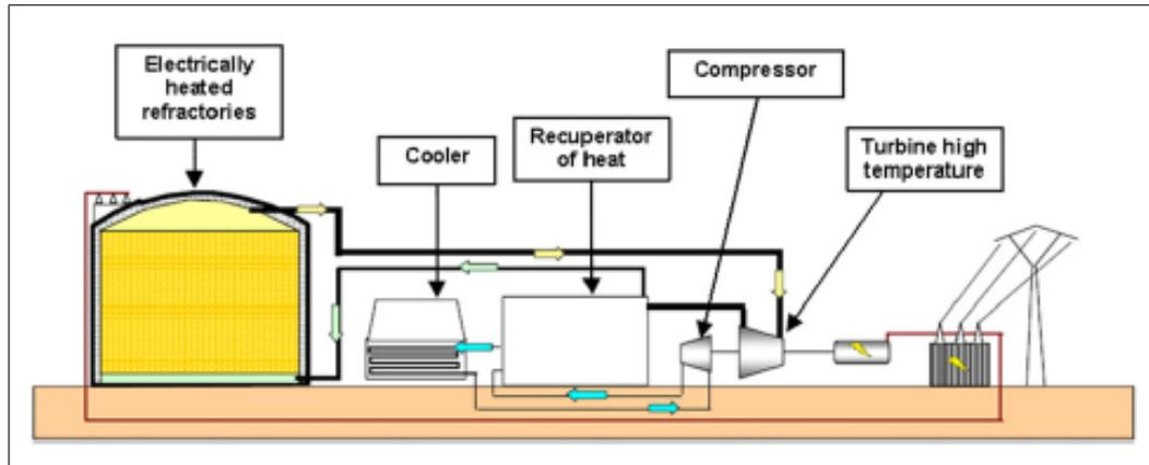
FIGURE 5.2. High-temperature heat storage with turbine (Ibrahim et al., 2008)
