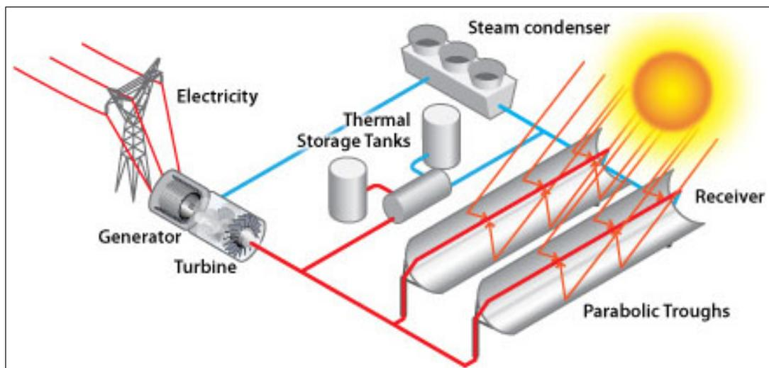
FIGURE 3.1. Parabolic Trough Energy Conversion Process(US DOE, 2010)
