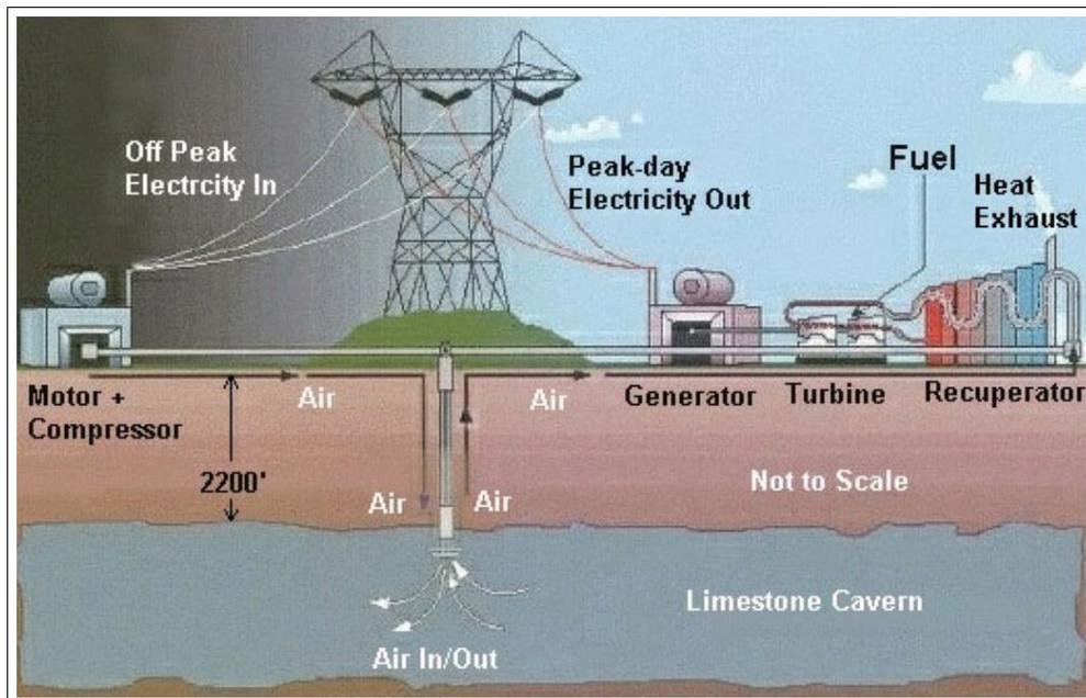
FIGURE 5.3. Compressed Air Energy Storage (Ibrahim et al., 2008)
