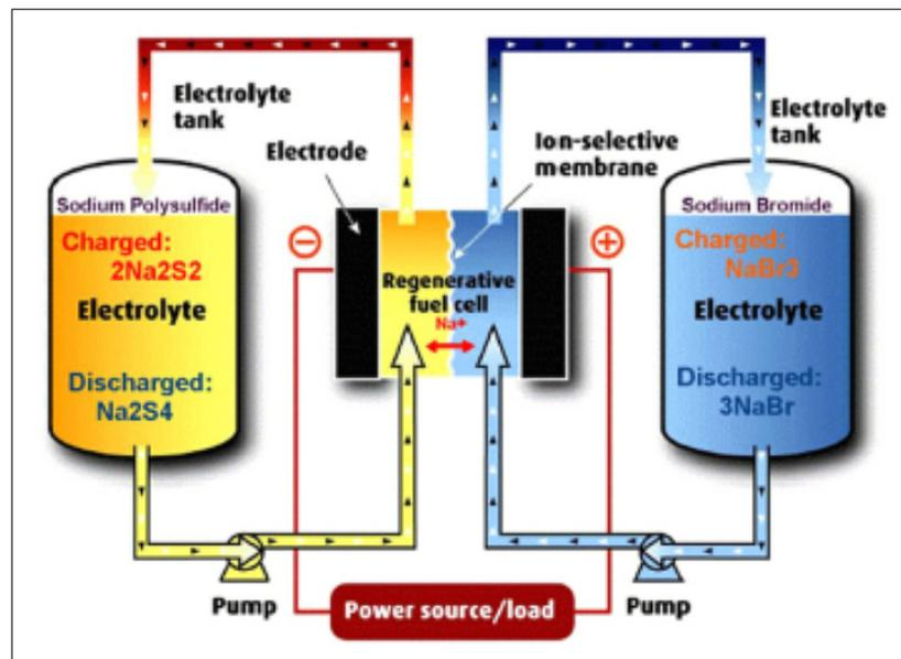
FIGURE 5.4. Flowbattery type FSB (Polysulfide Bromide Battery) (Ibrahim et al., 2008)
