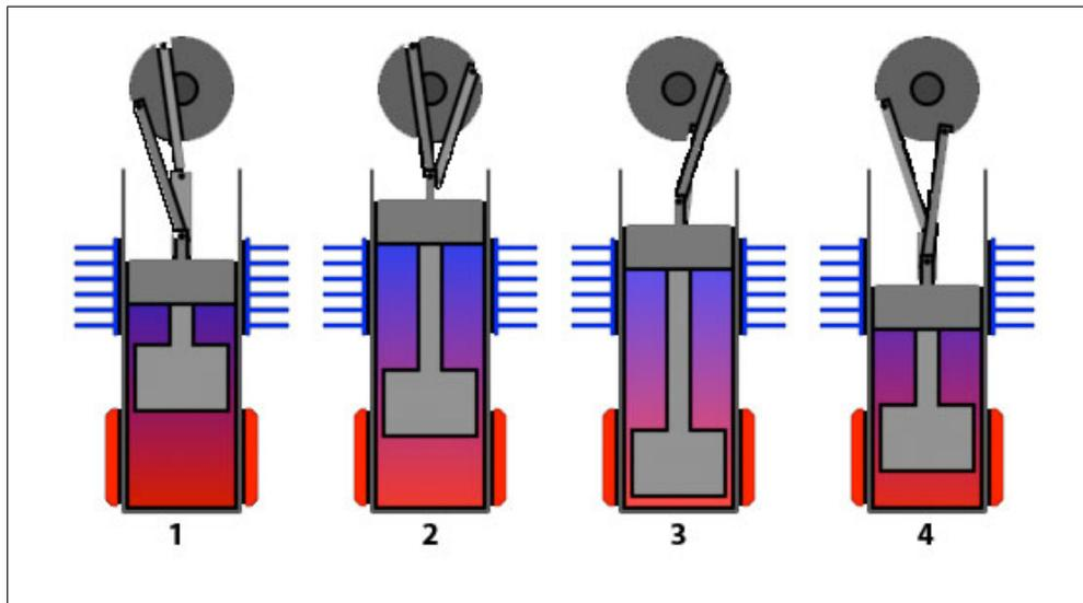
FIGURE 3.5. Stirling Engine Workflow Diagram (Wheeler, 2007)
