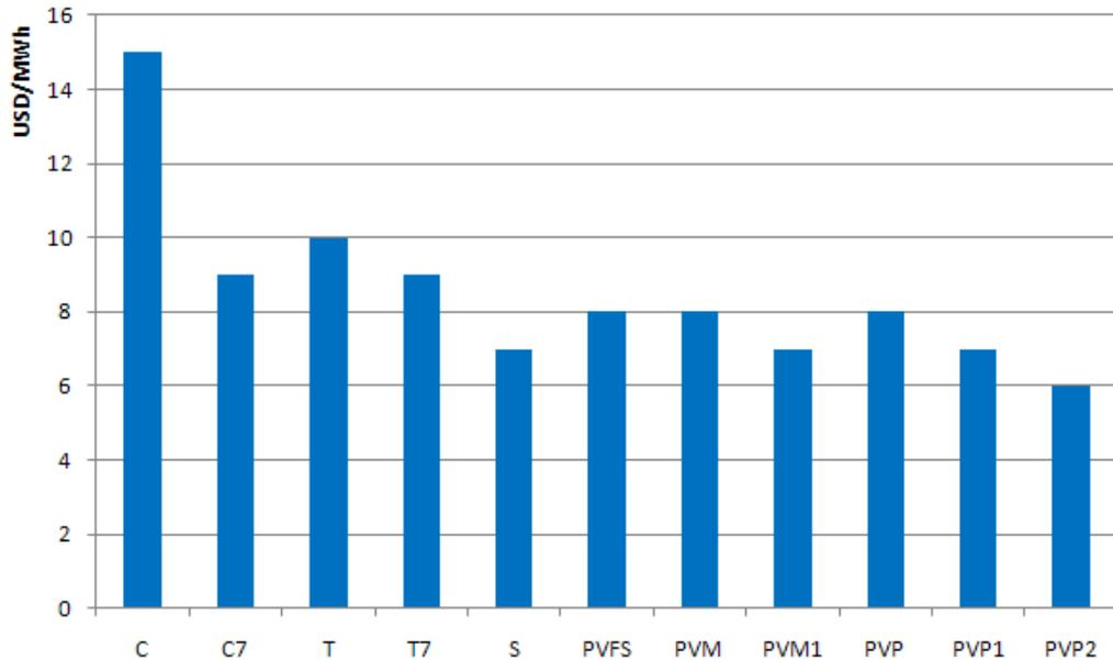
FIGURE 7.9. Operation and maintenance cost for a solar plant in Chile
