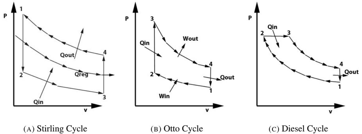
FIGURE 3.4. Comparison Between Different Engine Cycles
