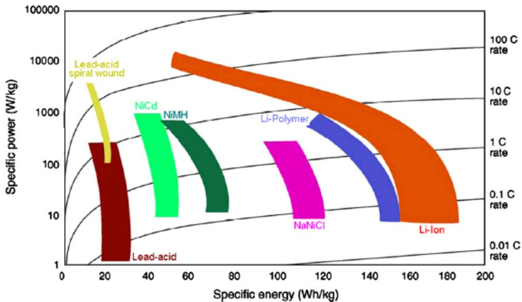
FIGURE 5.6. Different Electrochemical accumulators according to their energy densities and power (Ibrahim et al., 2008)
