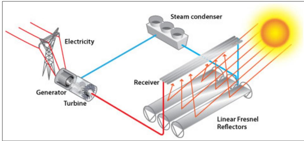
FIGURE 3.2. Linear Fresnel Energy Conversion Process (US DOE, 2010)
