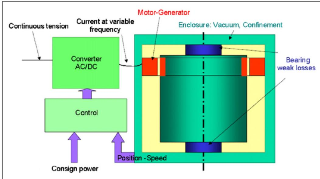
FIGURE 5.7. Flywheel Energy Storage System (Ibrahim et al., 2008)
