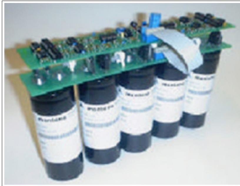
FIGURE 5.8. Supercapacitors assembled in series (Ibrahim et al., 2008)
