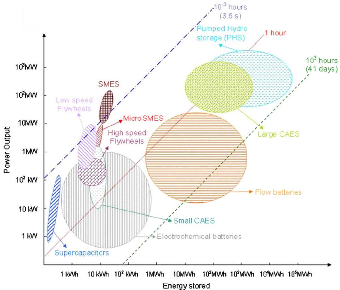
FIGURE 5.9. Energy Storage and Power Output for the Different Technologies (Ibrahim et al., 2008)
